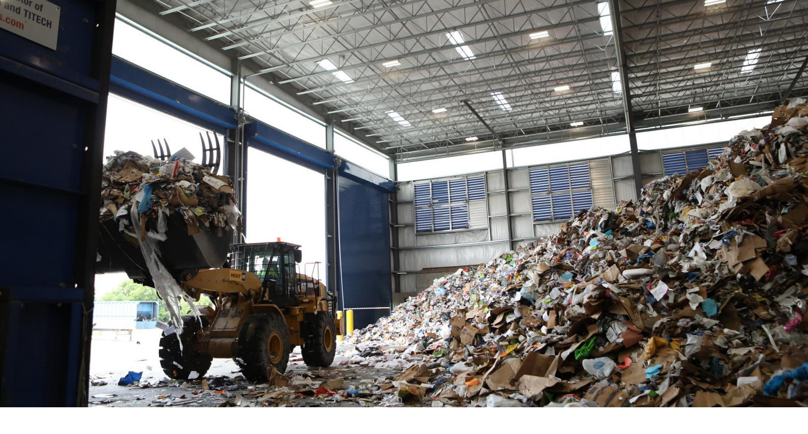
Trucks and forklifts deliver and move material on the tipping floor.
